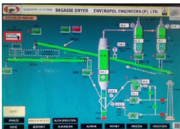
Fig. 4 DCS snap shot of Dryer in operation
